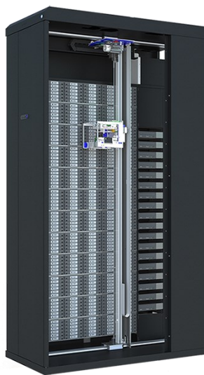
Figure 54. NETZON HDL 10368 holds 10368 discs enclosed in 864 cartridges and 36 parallel drives. [35]
