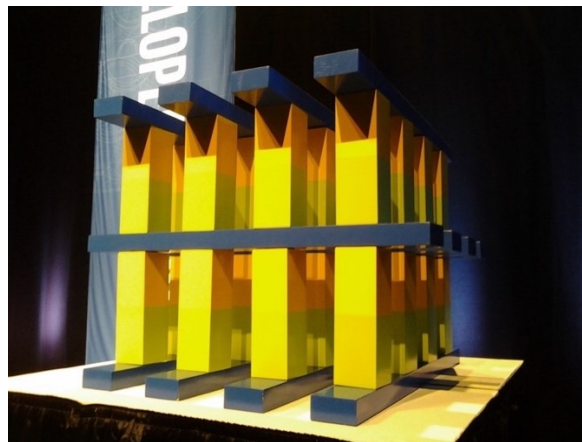
Figure 9. Physical Mock-Up of a 2-Layer 3D XPoint Memory Structure
